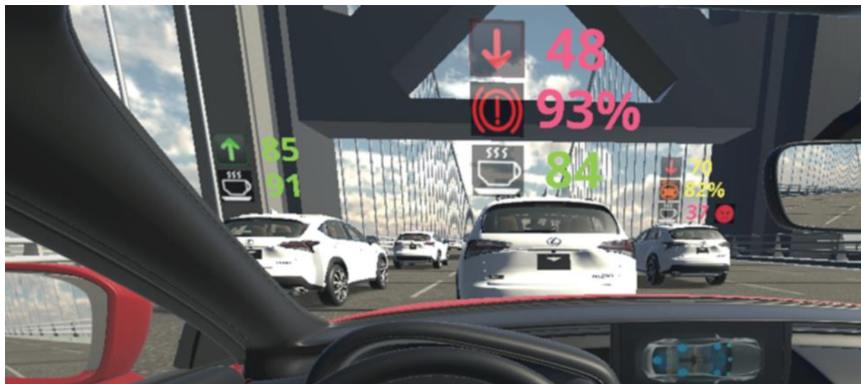
Figure 6: Prediction and guidance information received from the vehicle digital twin on the cloud is visualized through an augmented reality (AR) head-up display (HUD), which may include driving proficiency score and its trend, potential action (e.g., hard braking or lane change) and its possibility, as well the driving mood score 1
